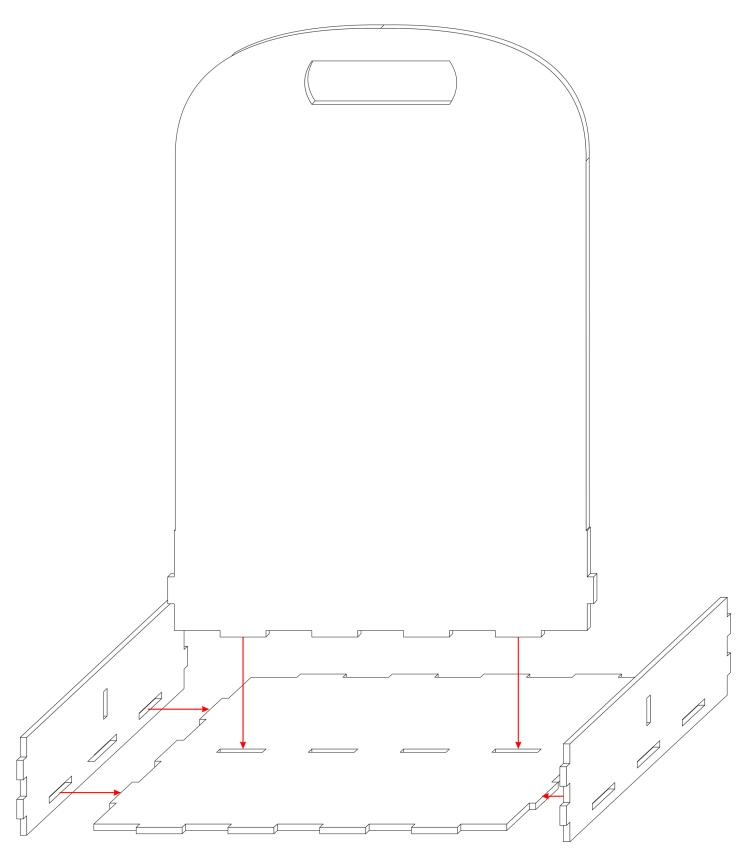
Start the bottom tray by gluing the divider/handle part first. Follow with the side elements. Clamp and leave to dry.
