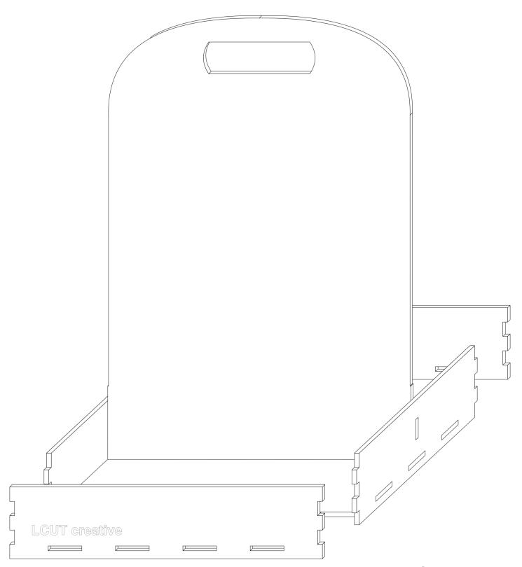
Finish off the bottom try by gluing the longer, front and back elements. Clamp and leave to dry.
